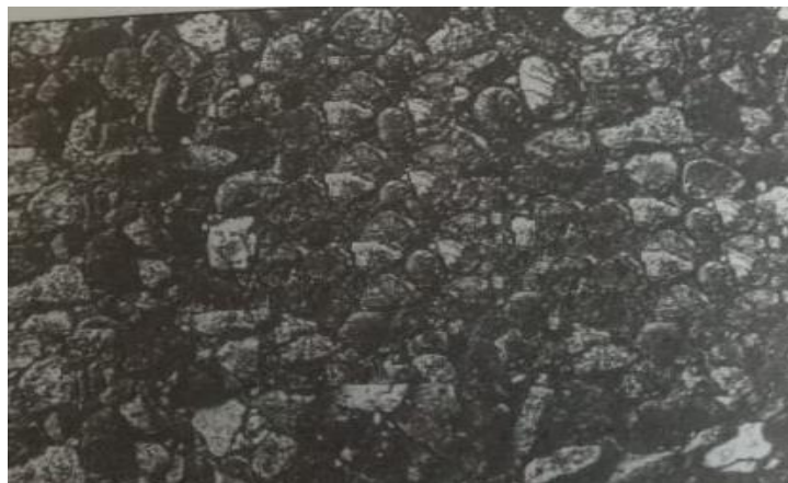
Gambar 3.22 Agregat Licin Sumber : Hardiyanto, 2015, 256
