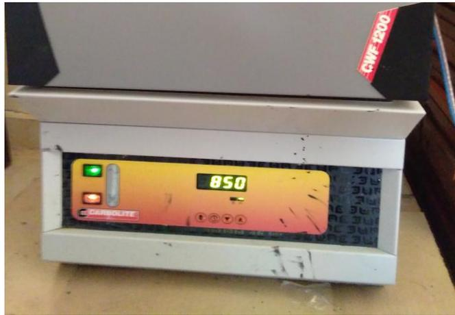
Gambar 3.5. Temperatur suhu oven 850 °C
