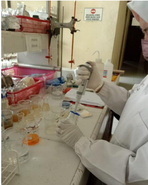
Pipet Larutan pereaksi asam sulfat 3.5ml kedalam tabung kultur
