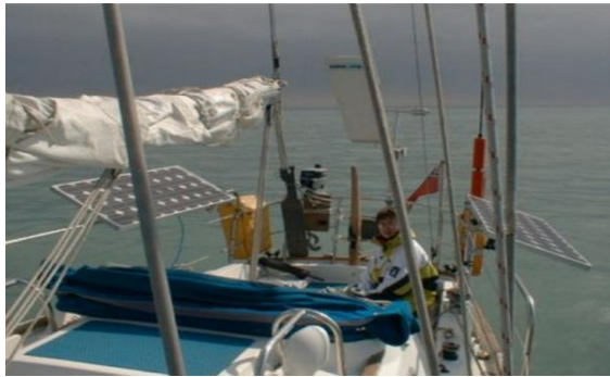
Gambar 2.3 Panel surya (photovoltaic arrays)
