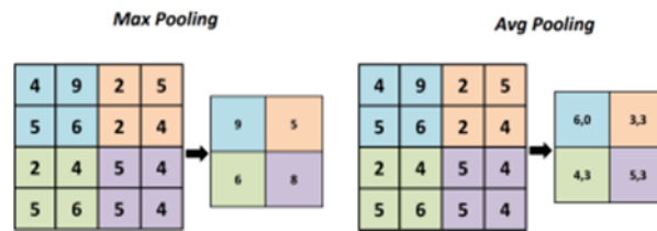
Gambar 2. 8 Max Pooling dan Average Pooling [14]
