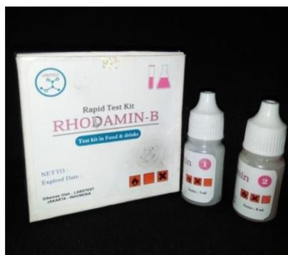
Gambar 3.3 Rapid Test Kit Rhodamin B
