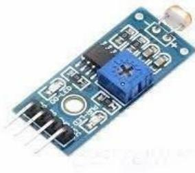
**Gambar 2. 5 Sensor Cahaya LDR (*Light Dependent Resistor*)**
