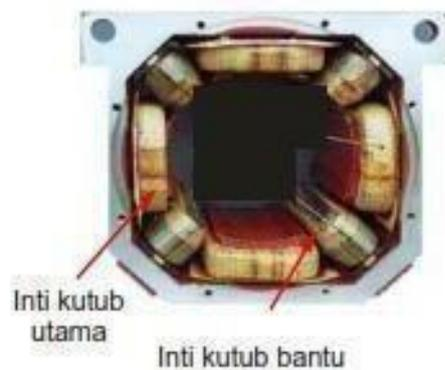
**Gambar 2. 4 Stator Mesin DC**
