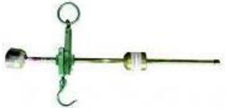
**Gambar 2. 2 Timbangan Manual (Pangkalan Getah Kumu Deli)**
