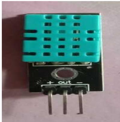
**Gambar 2.2 Sensor *DHT 11***
