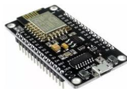
**Gambar 2.1 *NodeMCU ESP8266***
