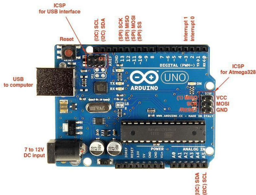
Gambar 2.2 Pin-Pin Arduino
