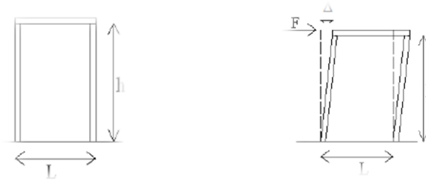
Gambar 3. 2 Perhitungan Drift Indeks
