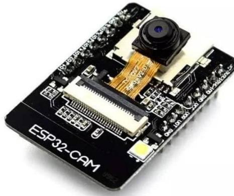
**Gambar 2. 1 Modul ESP32-CAM**
